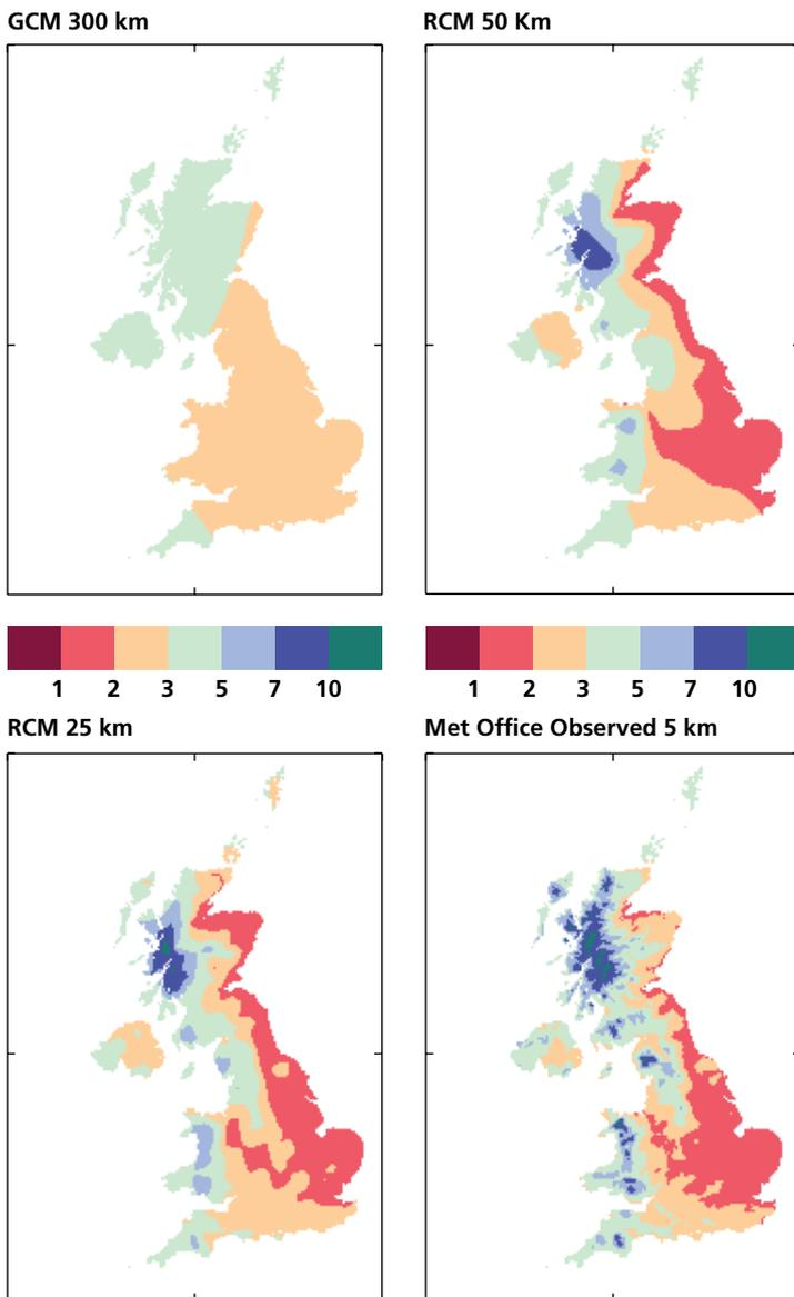
**Figure 5.1:** The distribution of winter precipitation over Britain (bottom right map) for 1961–2000, compared to simulations for the same period from a GCM (top left), and from two versions of the corresponding RCM at 50 and 25 km resolution, both driven with boundary conditions derived from analyses of observations. The GCM (inevitably) fails to resolve the observed spatial detail, whereas the RCM simulations show better agreement with increasing resolution.
