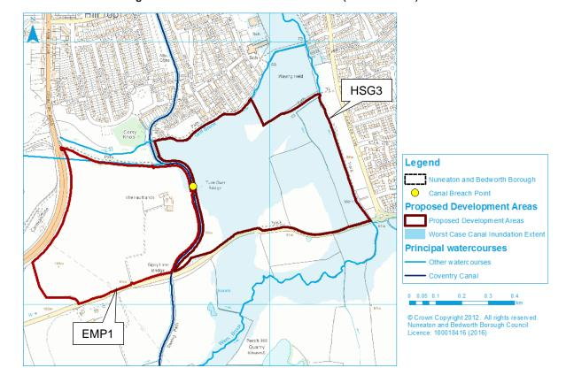
Figure 9-3: Canal inundation at Site HSG3 (Scenario Two)
