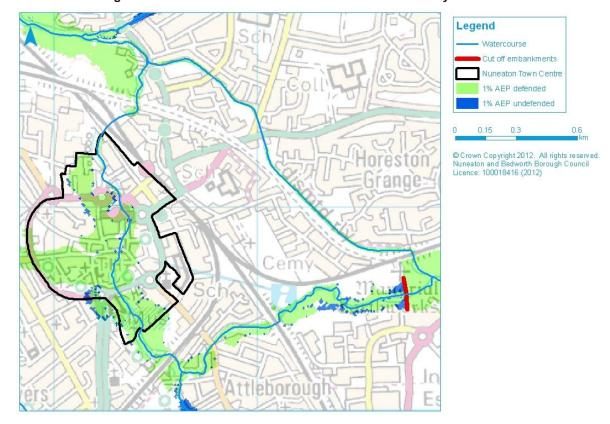
Figure 10-3: Removal of cut-off embankments in a 1 in 100-year event
