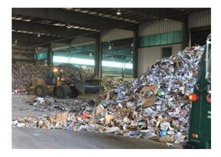
Waste is off loaded into the tipping bay, no need to tip at multiple bays
