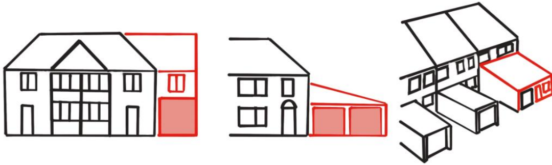
Figure 29: Extensions unsympathetic to the original roof form of the house
