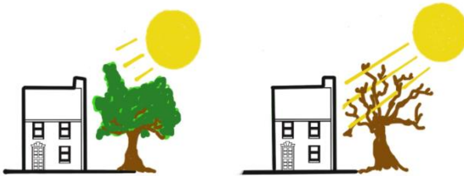
Figure 34: Tree function in Passive Solar Design
